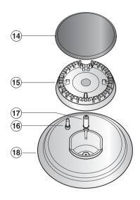
After cleaning the burner it must be reassembled in the correct order.
